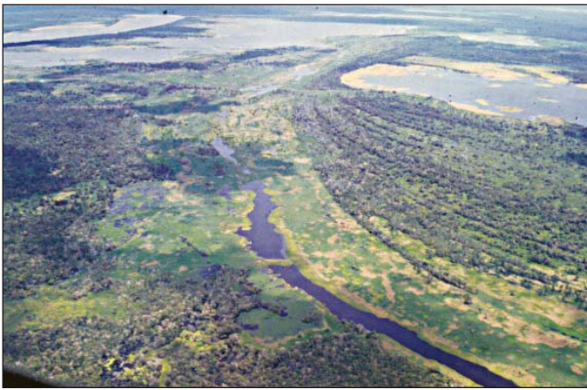
The Amazon floodplain near Manaus, Brazil. Nearly 100% of the area is inundated, despite the lack of visible open water. Furthermore, much of the flow occurs outside the channel (photo center), making a single gauge nearly useless for measuring discharge. A series of water surface elevation maps would show how the volume of stored water changes with time.
